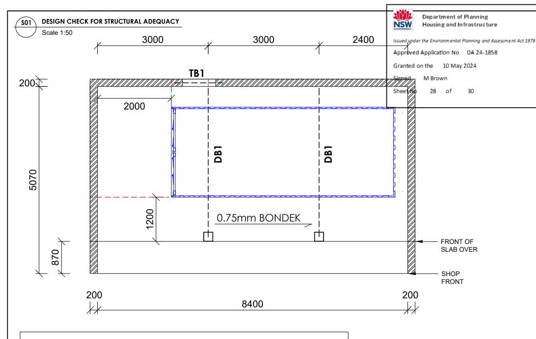
LOAD CHECK - PLACEMENT OF 'CONTAINER KITCHEN' OVER THREDBO VALLEY TERMINAL SKI TUNING SHOP.
